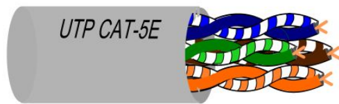
Figure 3. Category 5E UTP (Unshielded Twisted Pair) cable.
